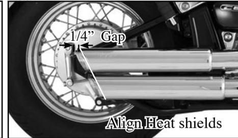
1. Install the bracket stamped 629-P, (supplied) to the motorcycle chassis using the 3/8" x 1" flange bolts, washers, and nuts (supplied) and tighten to factory specs (Figure 4).
