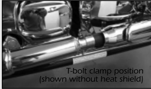
T-bolt clamp position (shown without heat shield)
