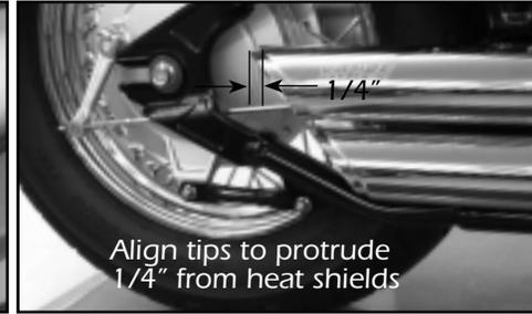
Align tips to protrude 1/4" from heat shields
